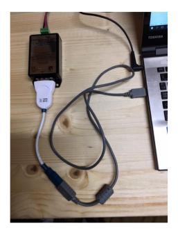
Connect the Serial USB interface to the Bus generator BG232/MT232 (can be a black or a white box) and the computer.
